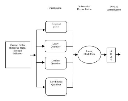
Figure 4: Different Quantization Schemes in Key Generation
