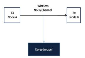
Figure 1: General concept of physical layer security
