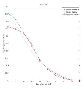
Figure 6: KDR and SNR for different Quantizers
