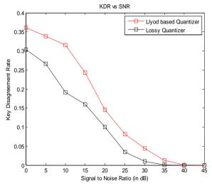
Figure 7: Graph between KDR and SNR for LQ and LYQ
